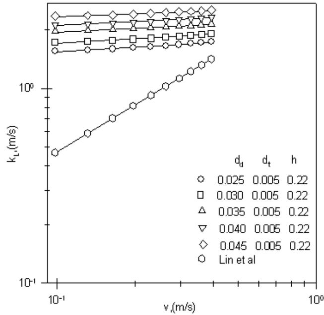
Figure 5: Variation of mass transfer coefficient with velocity
