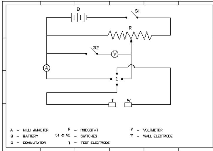
Figure 4: Circuit Diagram
