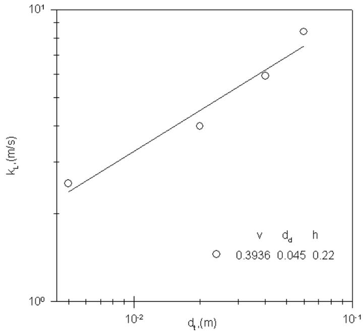
Figure9: Variation of mass transfer coefficient with disc thickness
