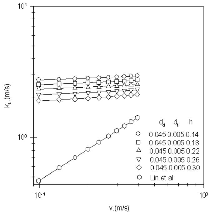
**Figure 11: Variation of mass transfer coefficient with velocity of electrolyte**
