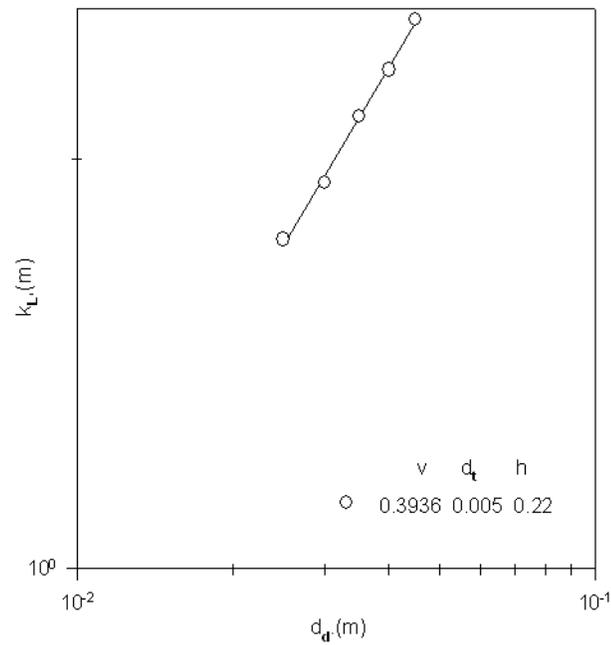
Figure 6: Variation of mass transfer coefficient with disc diameter
