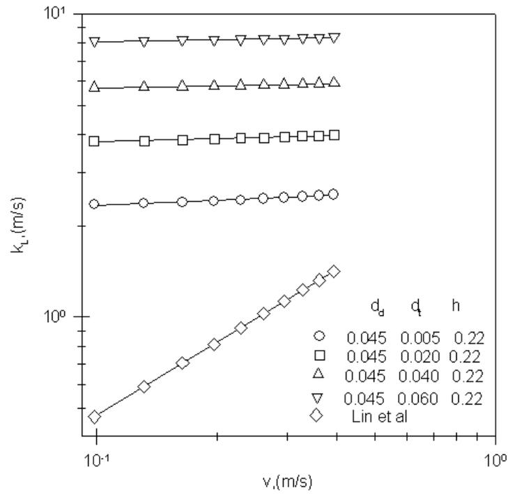
Figure8: Variation of mass transfer coefficient with velocity
